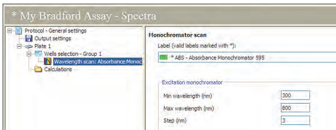
Figure 2. EnVision Manager settings for running a Wavelength Scan operation. The scan range and step size are entered in nanometres to the protocol. A baseline is required to be run through Wizard for absorbance wavelength scans.
